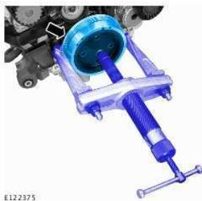
8. **⚠ NOTICE:** Make sure that the installation marks are aligned.
